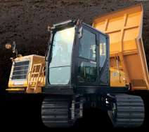
MST-70CR Max Payload 7t Tier4 Final / EU Stage V
