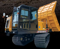
MST-1000VDR Max Payload 5.5t Tier4 Final / EU Stage IV
