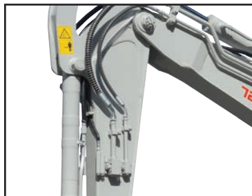
Auxiliary Hydraulic Lines
