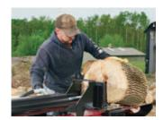
**DURABLE DESIGN**Strong I-beam and 9" solid steel splitting wedge add to the durability of the machine.
