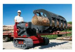
**GRAPPLE RAKE** (MODEL 22577) Grab, drag, lift and place brush and debris easily with up to 3,000 lbs (1,361 kg) of clamping force at the tine tips.
